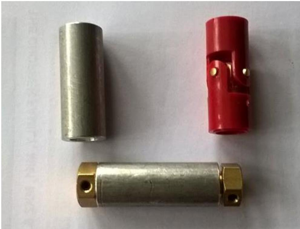
This is simply a piece of ½ inch diameter aluminium. The length being identical to the red plastic joint and the ends are drilled so that the two brass inserts are a “snug fit” i.e. they fit into the aluminium with just finger pressure and can be removed in the same way. The brass inserts providing the interface between the motor and propshaft.
