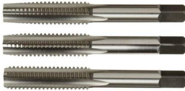
In descending order Taper, Second and Plug
