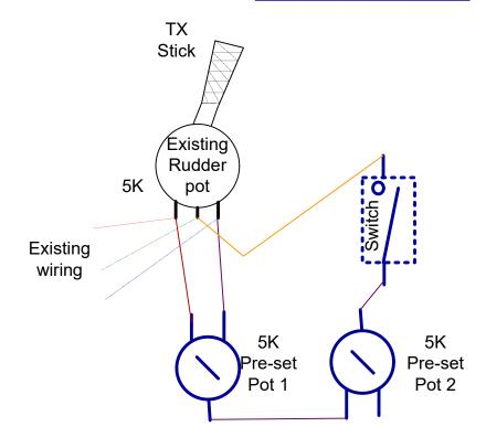
Add a dual rate switch will give you more control. Set pot 1 first to centre the servo then pot 2 to limit the rudder or throttle as required.
