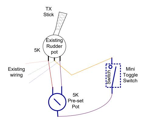
Add a single or dual rate switch to the transmitter to limit the rudder or throttle as required.
